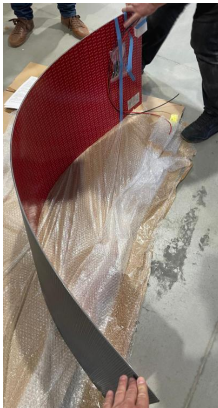
Fig. 14 - Activesol NAVY-BLUE panel with integrated 3M VHB GPH-110F tape
