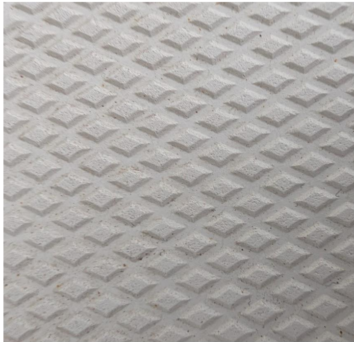
Fig. 3 - Deep anti-slip surface structure
